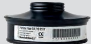
SR 710 particle filter P3 R is a mechanical particle filter of class P3 R with an extremely high efficiency (> 99.997%) and an active area of 13 dm<sup>2</sup>.
