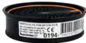
SR 510 P3 R is a mechanical particle filter with extremely low breathing resistance. SR 510 offers protection against all types of particles (dust, smoke, mist, spray, asbestos), as well as bacteria, viruses and radioactive fallout. Filtering efficiency more than 99.997%. SR 510 is used for all protective filters in Sundström Safety's programme. If gas/vapour and particles occur simultaneous-ly, a particle filter is combined with a suitable gas filter.
